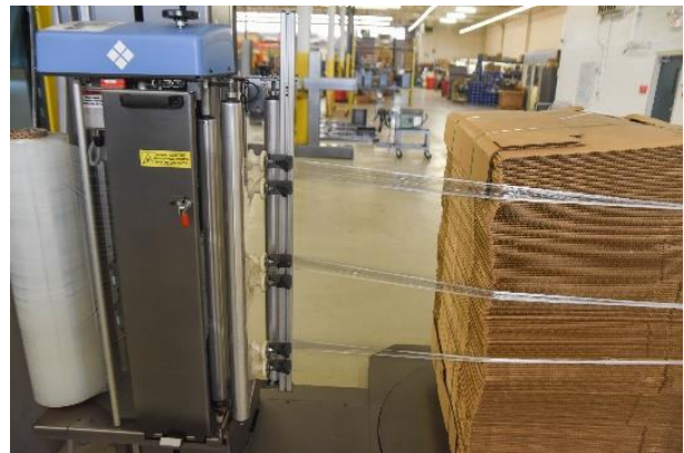
Shown splitting 30" film into (3) 10" bands
