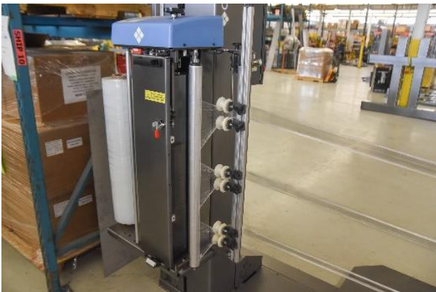
Shown splitting 30" film into (3) 10" bands
