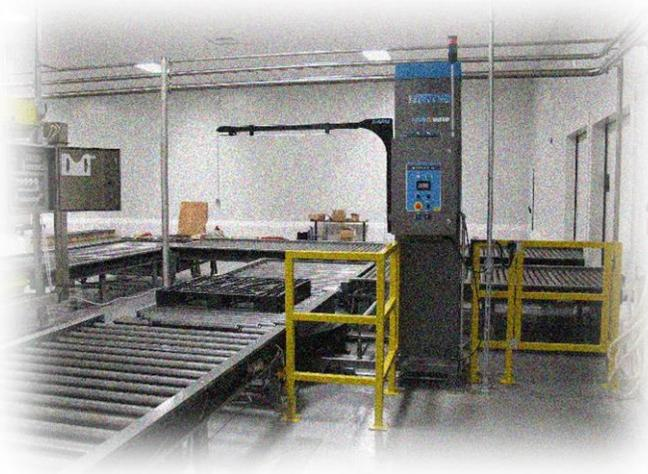
**SYSTEM CONFIGURATION** – Designed to be installed with existing product flow and conveyor layout design. Whether In-line or off-line, the automation package is designed to be in-line with conveyors using interface relays/logic or off-line standalone system using a wireless cycle start remote.
